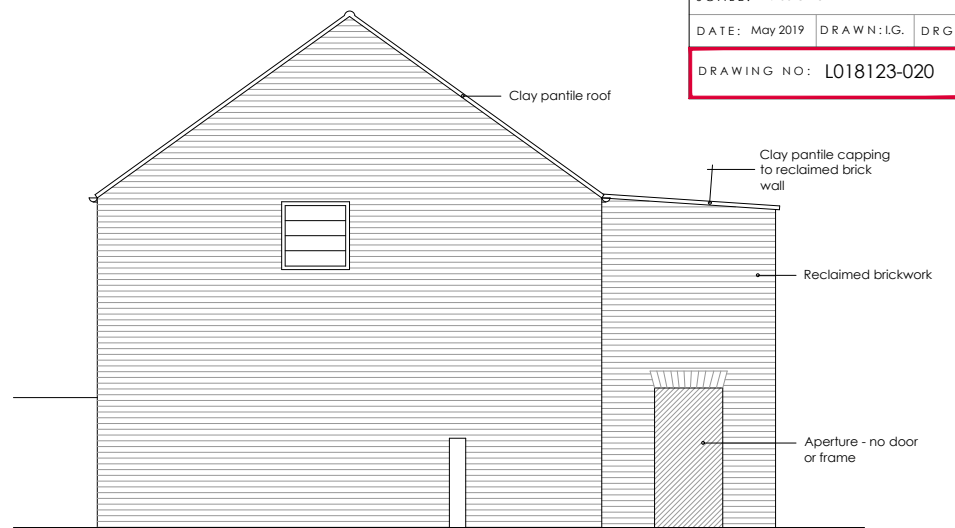
Proposed Front and Rear Elevations ( Ancillary Accommodation ) 1:100
